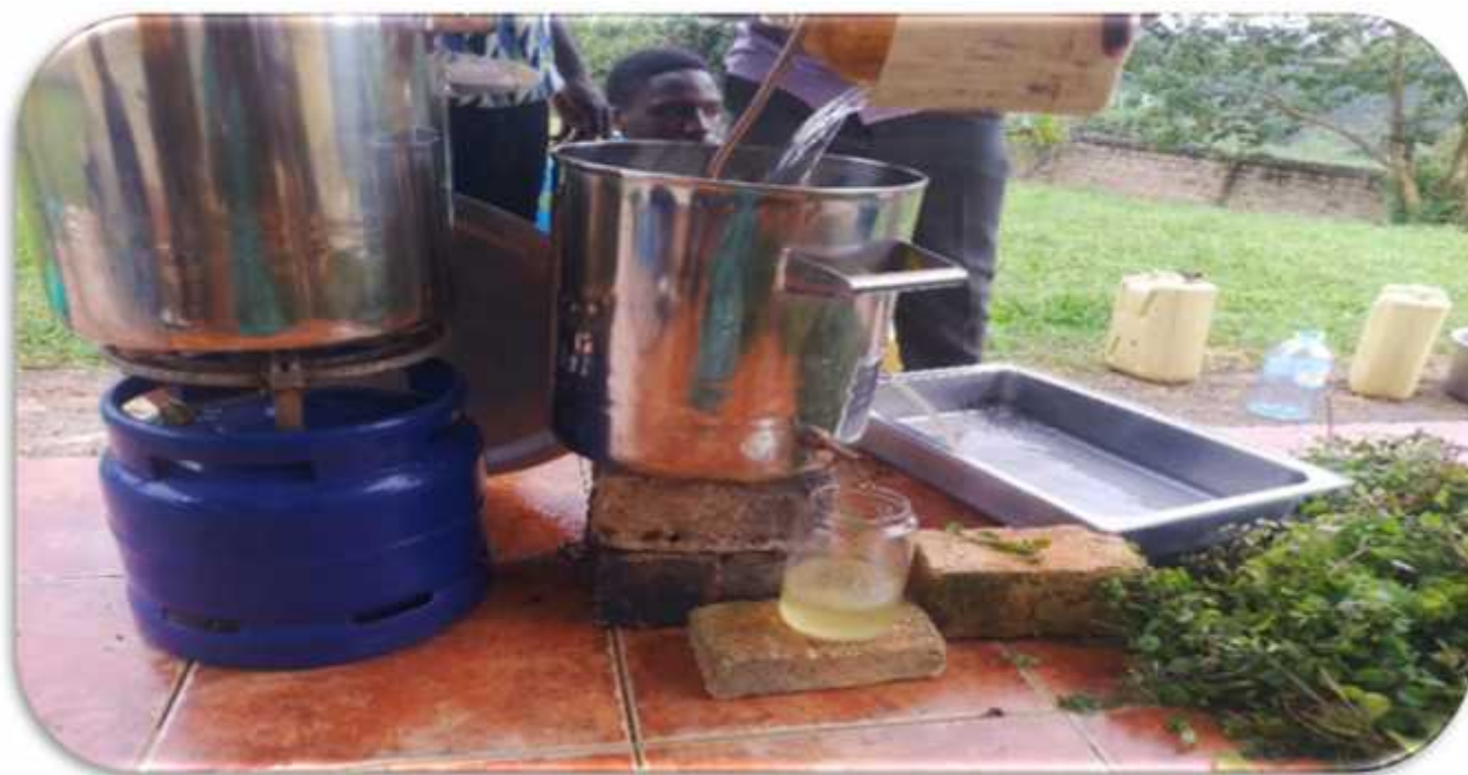
The condenser being filled with cold water after removing the hot water
